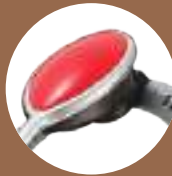
Infrared Sensor Maintains Scalp Temperature
